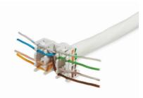
Lay the wires to their correct positions based on the color code (T568A/T568B).
